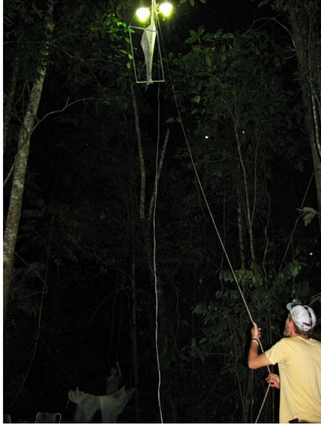
Figure 5. Suspended light trap during field work in Itapiranga
